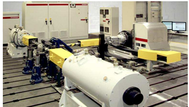
Figure 5 Transmission test stand with two Wheel Dynos
